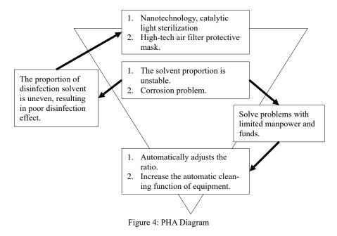
The PHA plan for the design of epidemic prevention, sterilization and disinfection channels is shown in Table 1. In this study, the most suitable improvement plan for this study is the automatic allocation ratio of the machine and the addition of the automatic cleaning function of the equipment.
