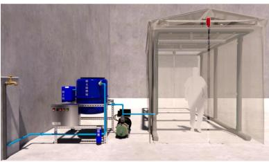
Figure 8: Schematic Diagram of the Improved Disinfection Channel
